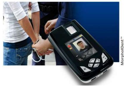
DPS)-compliant ANSI/NIST file and submits the search request to the NC-DPS AFIS system for identification. Results are returned to the MorphoMobile application screen and to the MorphoIDent for notification and positive identification, if available.
