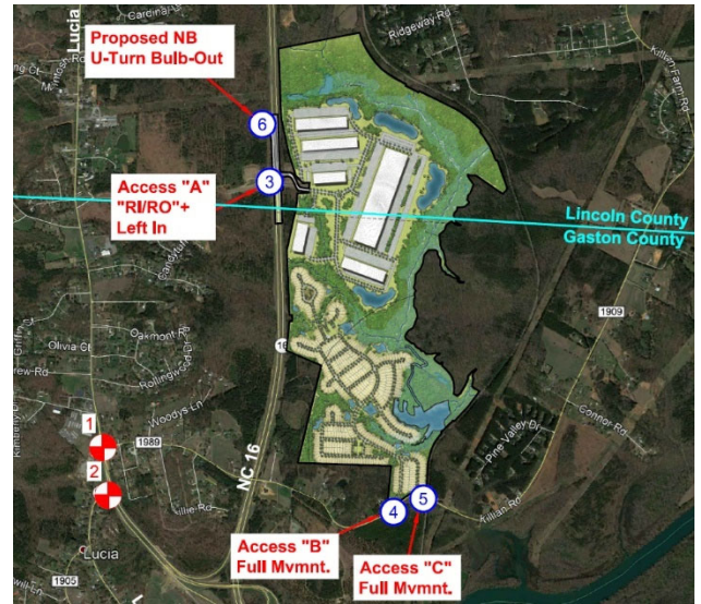
Figure 1 - Access Points for East Side of the Development - the Industrial site will only have access off if NC 16 on the Lincoln County side of the County Line
