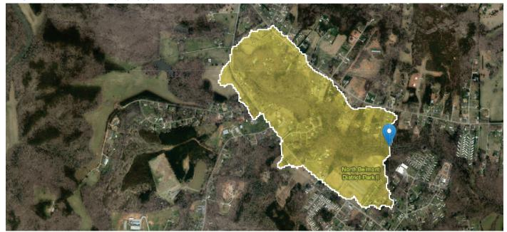
Delineation for Stormwater Wetland to treat runoff from North Belmont Park. Draining to the proposed wetalnd is 37.5 acres
