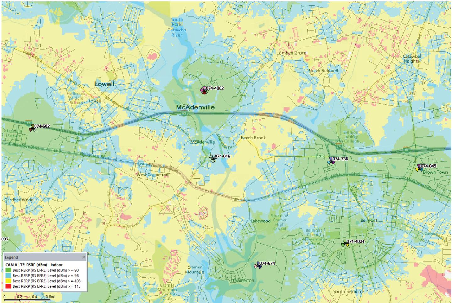
AT&T could not meet their coverage and objectives if we lowered our RAD height to 195' which are to provide & enhance the coverage along I-85 and also provide outdoor/indoor coverage to residential and businesses around the town of McAdenville. Refer to **Figure 5** which shows coverage with proposed site 074-4082
