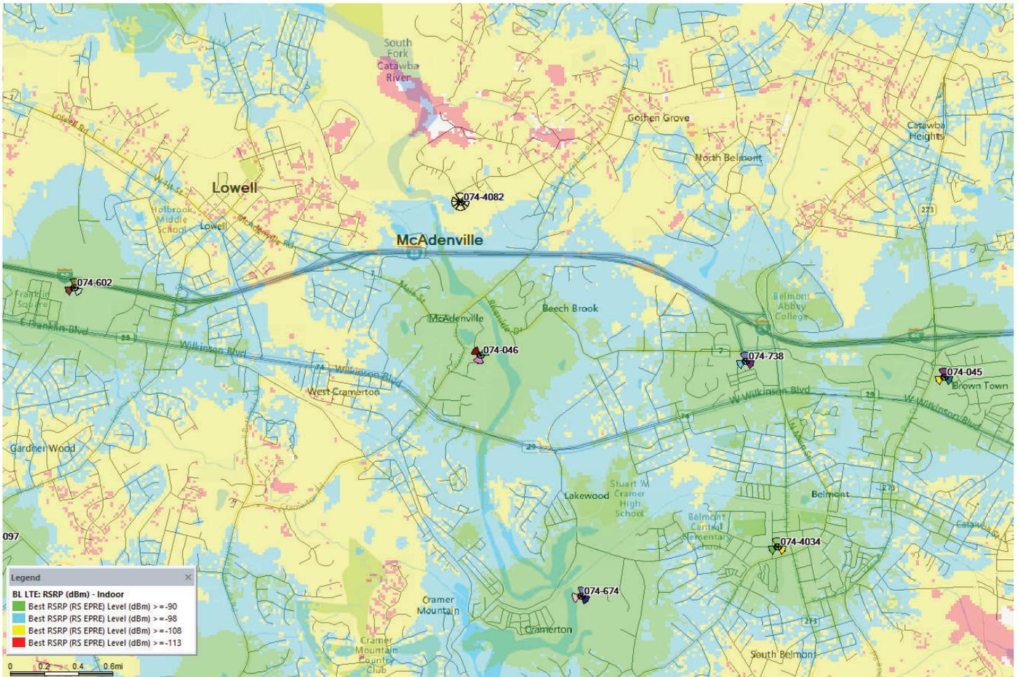
Coverage after Crown site was removed. Refer to **Figure 3**, which shows loss of coverage without existing site 074-046.
