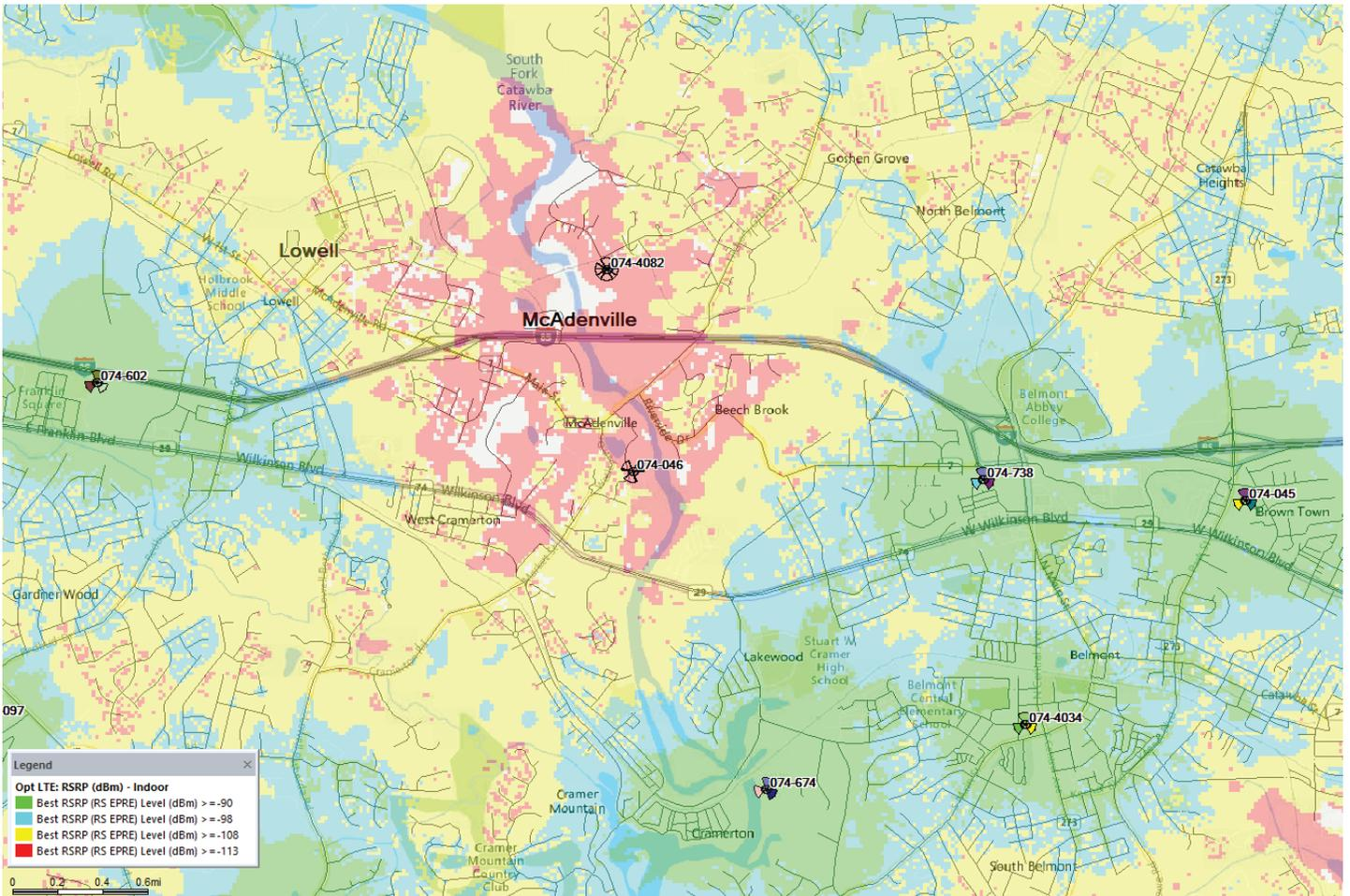
With the addition of the relocation site 074-4082, AT&T Mobility will provide & enhance the coverage along I-85 and also provide outdoor/indoor coverage to residential and businesses around the town of McAdenville. Refer to **Figure 4** which shows coverage with proposed site 074-4082
